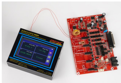
Example of printed circuit board strain measurement
